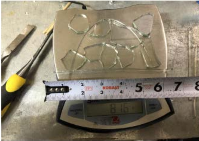
Photo No. 1 Impact Specimen No. 3 Failure
